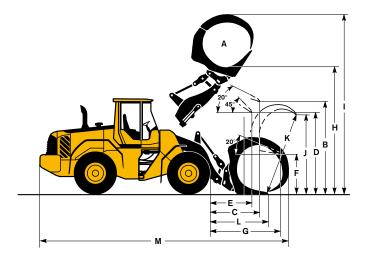
L110F Sales code: WLA80832 Operating weight (incl. logging cw 680 kg/1,500 lb): 19 820 kg (43,710 lb) Operating load: 5850 kg (12,900 lb) L120F Sales code: WLA80832 Operating weight (incl. logging cw 680 kg/1,500 lb): 20 600 kg (45,420 lb) Operating load: 6400 kg (14,110 lb)
