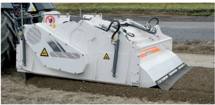
Their design prevents the side plates from being pulled through the soil, sapping power needlessly
