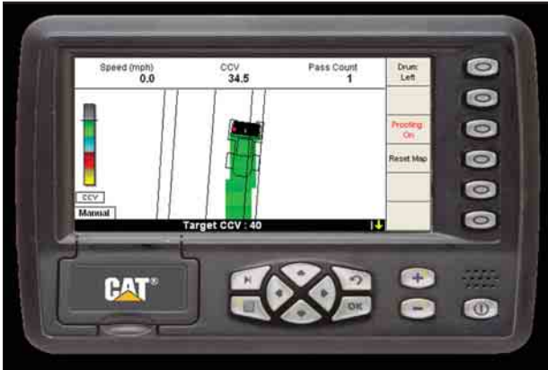
The display provides the operator with compaction data as it is measured.
